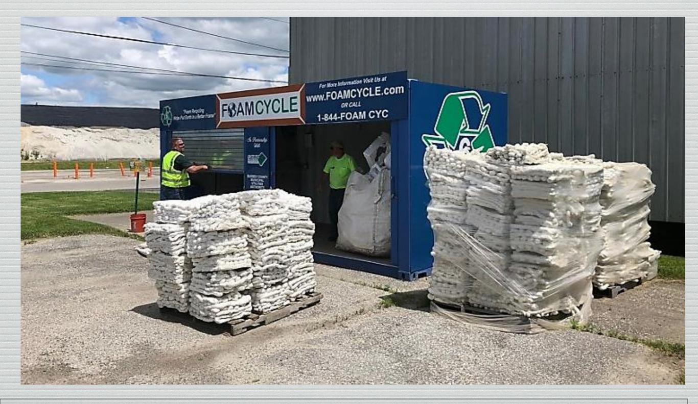
Foam Packaging is made up of 98% air & 2% polystyrene plastic Each Foam Cycle system is equipped with a foam densifier machine capable of removing all of the air and extruding the 2% polystyrene plastic called ingots.
